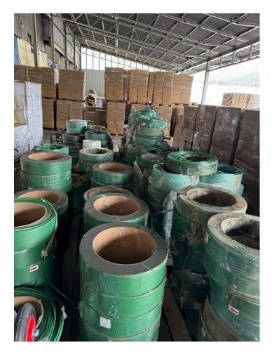
PET STRAPS 12 X 0.6MM/406 - 2500M - STRENGTH 310KG - FLOODED - 61 UNITS
